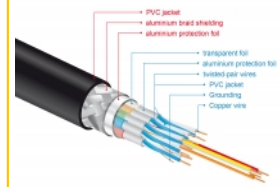
Triple shielding for lossless signal transfer
