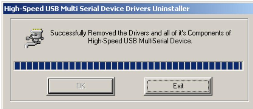
The driver can also be uninstalled from **Control panel – Add / Remove Programs**. Select the “High-Speed Multi Serial Compound Device” from the Add / Remove panel and click on “**Remove**” option. This will remove the MCS7840 device driver from the PC.
