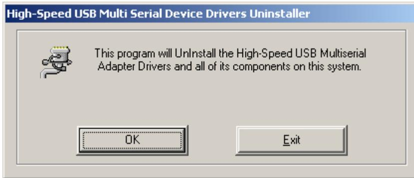
Use the “**Exit**” button to complete the Uninstaller utility. No need to restart the PC, unless prompted by the OS.
