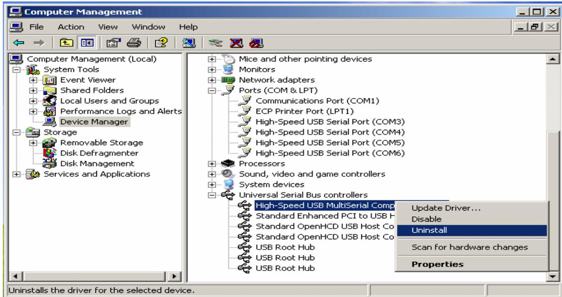
The OS will prompt the user whether to uninstall the device from the system. Click on “OK” to uninstall or “Cancel” to terminate the un-installation.
