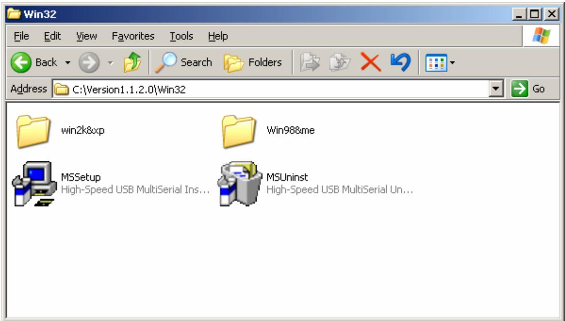
Use “**MSSetup.exe**” utility to install the driver. Double click on the utility to start the installation process. Press “**Install**” button to install the drivers for High-Speed USB Multi serial Device.
