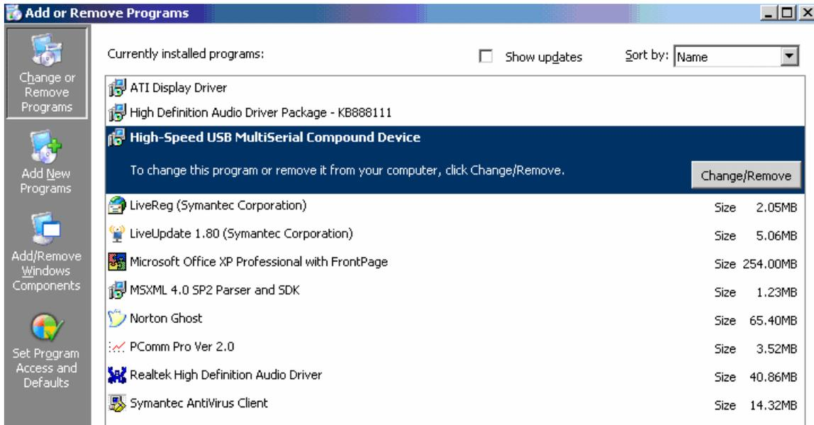
The MCS7840 device driver can be un-loaded through “**Device Manager**” as well. Go to Device Manager, Select High-Speed USB Multi Serial Compound Device from the Universal serial Bus controllers, Right Click on it, Select “**Uninstall**” as shown below.
